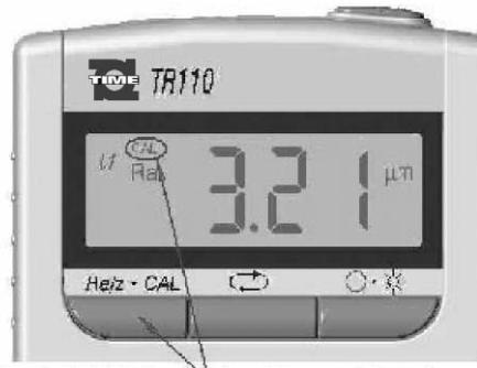
Press the Left Key and Middle Key to adjust the displaying value to the value indicated on the standard sample plate (Refer to picture 10).
