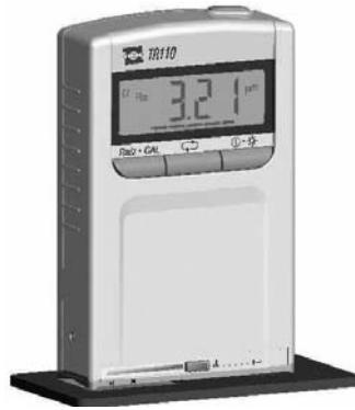
When the tester is under non-measuring status, keep pressing the Left Key more than 2 seconds, the tester will enter the status of Calibration. (Refer to picture 9)
